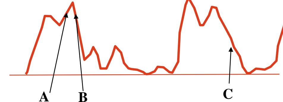
$$I_A \sim I_B \neq I_C \quad \left\{ \begin{array}{l} \langle I_A I_B \rangle = \langle I_A^2 \rangle = 2 \langle I \rangle^2 \\ \langle I_A I_C \rangle = \langle I_A \rangle \langle I_C \rangle = \langle I \rangle^2 \end{array} \right.$$
